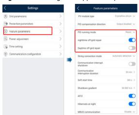
Figure D-1 Setting PID suppression parameters
