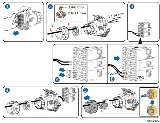
Figure 5-23 Connecting the cable
