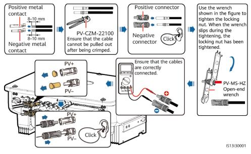
Figure 5-8 Connecting the DC power cable
