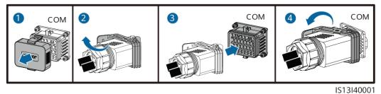
Figure 5-18 Securing the signal cable connector
