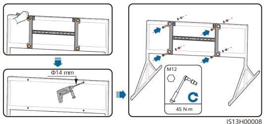
Figure 4-11 Securing the mounting bracket
