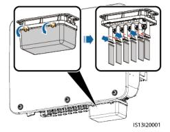
**Step 2** Connect the AC output power cable (using a five-core cable as an example).
