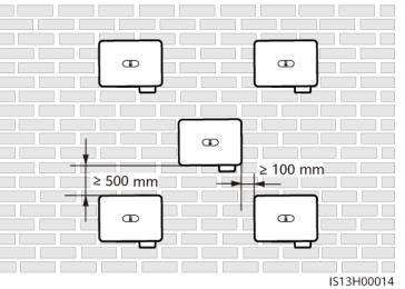
Figure 4-5 Three-layer triangle installation (not recommended)
