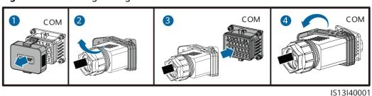
Figure 5-22 Securing the signal cable connector
