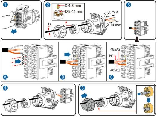
Figure 5-19 Connecting the cable
