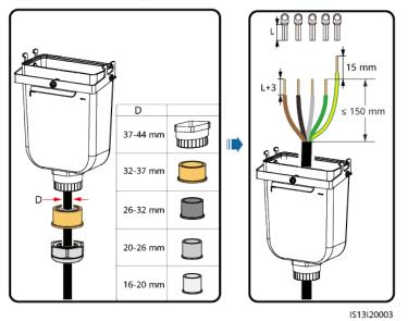
**Figure 5-6** Connecting the AC power cable
