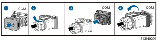
Figure 5-20 Securing the signal cable connector
