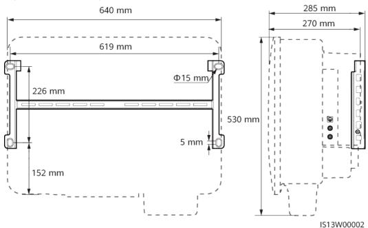
Figure 4-10 Mounting bracket dimensions
