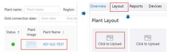
Step 2 Log in to https://intl.fusionsolar.huawei.com to access the WebUI of the FusionSolar Smart PV Management System. On the Home page, click the plant name to go to the plant page. Select Layout. Choose Generate Layout, and create a physical layout as prompted. You can also manually create a physical location layout.
