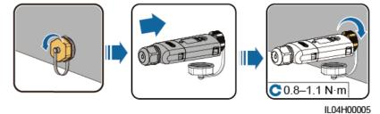
WLAN-FE Smart Dongle (FE Communication)
