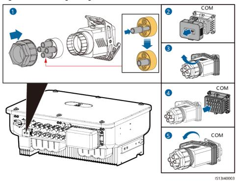
Figure 5-13 Securing the signal cable connector
