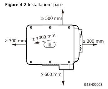
• When installing multiple SUN2000s, install them in horizontal mode if ample space is available and install them in triangle mode if no ample space is available. Stacked installation is not recommended.
