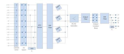
Figure 2-6 Schematic diagram
